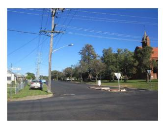
The power pole located on the south-western side of the intersection has a number of "scars" from where large vehicles have contacted with the outside edge of the pole. It is assessed that the pole is not in the best of condition however, it is considered that if a replacement pole was installed, it too would quickly become scarred. It would also be very difficult to relocate the said pole because of the four-directional multiply power lines in the vicinity.
